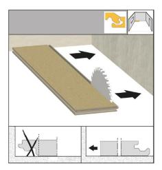
Remove the tongue from the first row of panels and place the trimmed side against the wall.
