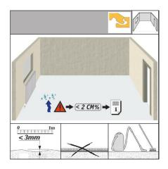
The substrate must be free of cracks, clean, tension/pressure resistant and permanently dry (VOB, part C, DIN 18365). The flatness of the substrate must not vary by more than +/-3 mm over 1 m (DIN 18202).
