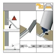
Where pivoting is not possible (e.g., under door frames and radiators), remove the cheek locking pin from the bottom groove using, for example, a chisel.
