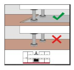
Fitted kitchens and built-in cabinets must be assembled prior to installation. Installation over flooring is not permitted.
