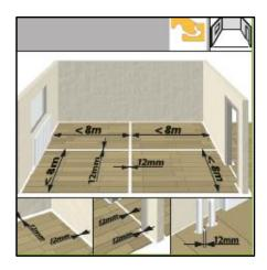
The largest possible continuous installation area is 8 m in the direction of the width of the board and 8 m in the direction of the length of the board.
