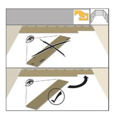
Before installation, check the boards for any defects. Boards with minor damage can be installed in areas where they should be cut anyway.
