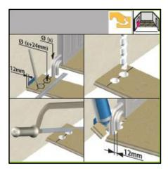
If, for example, heating pipes protrude from the floor, first cut the board to the right length. Then lay the board piece next to the actual location and measure and mark the recesses with the bending rule. Again, don't forget to leave a gap of at least 12 mm around the expansion joint. You can now drill the marked areas. Then saw the board to size. Then place it behind the heating pipe and join it back to the board
