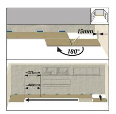
Turn the last board in the row 180° and lay it next to the existing row, decorative side up (take into account the distance from the wall at the end). Then mark the board and saw it.
