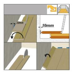
For the last row of panels, the boards must be placed exactly on the second to last row. Using a leftover piece (original width), transfer the distance to the wall to the board. The board is then cut lengthwise. Note the minimum distance.
